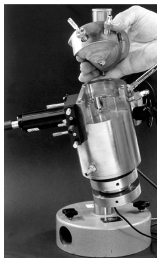
The pressure Jump Machine can reach pressures of up to 500 bar in 50 microseconds, 400 times in a minute forcing a protein to fold and unfold quickly.
